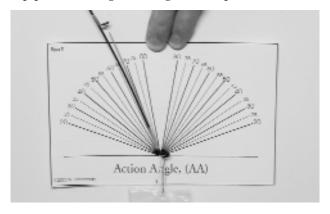
4. Making sure the AA chart base line is level, read the scale value indicated by the free end of the pointer and record that value as AA.
