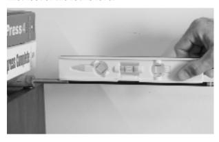
2. Measure the height of the horizontal rod butt (e.g., 64 inches). Ignore any tip droop.
